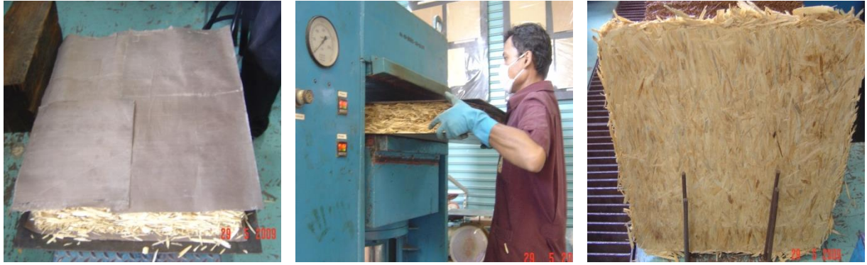
Figure 2. Production of Oriented Strand Board (OSB).
